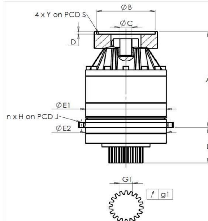
General tolerance: Js13 Cmm Automatic / manual coordinate-measuring machine µm Micrometer Cr Calliper rule Di Dial indicator Pg Plug gauge
